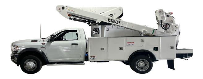
We are pleased to quote the VERSALIFT VST-40-I, insulated 40ft. 4 in (12.3 m) telescopic aerial platform lift, 45ft. 4 in (13.8.0 m) working height with a horizontal reach of 30 ft.2 in. (9.2) and to include the following items:
